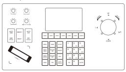
[PT Speed]: Twist the Speed Control knob in to cycle to increase or decrease the PT Speed. PT Speed Range: 1-8.
