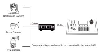
Connect the camera and joystick controller in the same LAN and ensure their IP address in the same network segment, such as 192.168.1.123 and 192.168.1.111 belong to the same network segment, while 192.168.1.123 and 192.168.0.125 do not belong to the same network segment, so you need to modify the joystick controller or the ptz camera IP address. The joystick controller gets its IP address dynamically.
